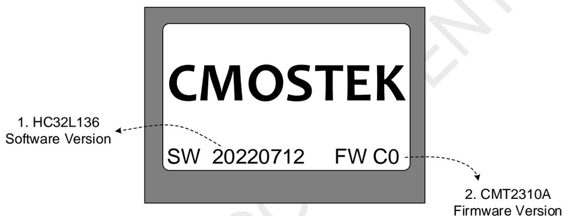
**Figure 2-1. Startup Interface (After inserted CMT2310A-EM)**
