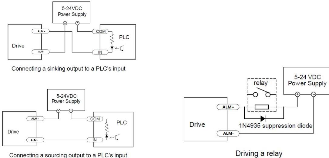
**Figure 6** Fault Connection
