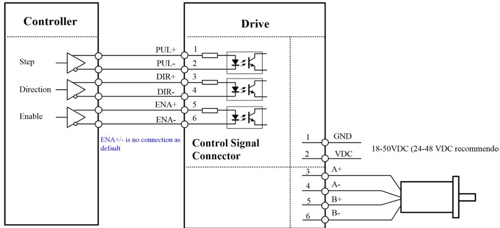
Figure 8 Typical Connections
